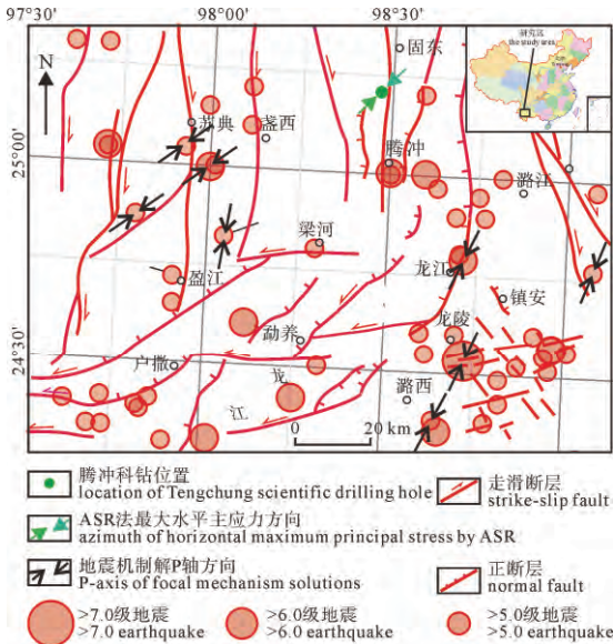
图 4 最大水平主应力方向与震源机制解的 p 轴方向比较( p 轴方向据吴中海等, 2013 修改) Fig. 4 The horizontal maximum principal stress from ASR And P-axis of focal mechanism solutions (P-axis is from WU et al., 2013)
